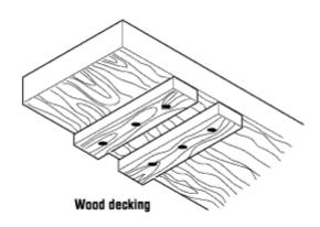
Only cleat planks at the ends to prevent lengthwise movement. Wiring down planks can
