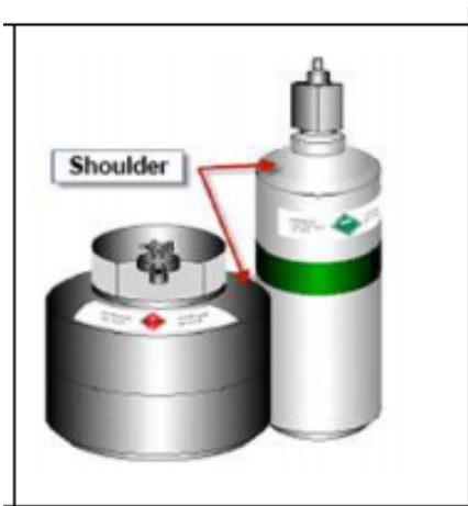
Figure 3: Labels on cylinders. Image from Alberta EDGE (Environmental and Dangerous Goods Emergencies), Alberta Transportation
